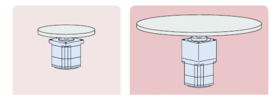
Increasing the size and weight will increase the inertia of the load and the torque required to move the load. Gearing is a great option for overcoming large inertia loads as it will decrease the reflected inertia on the motor by the gear ratio squared.
